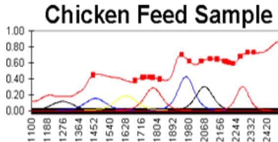
To create a calibration, samples are chosen which are representative to the samples that will be analyzed. There may be as few as 60 samples or there could be several thousand. These samples are analyzed in the NIR, and the spectra stored. The samples are then sent to have the reference analysis performed on them. These are termed calibration samples. We will use 60 sample analyzed for protein content and scanned on a NIRSystems model 5000 for this example.
