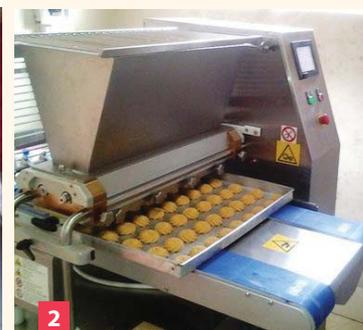
Fig. 2 Biscuits being shaped and formed (credit J. Low)
