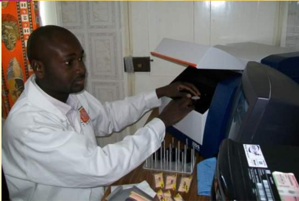
Near Infrared Spectrometer enables rapid (2 minutes) assessment of major macro- and micronutrients
