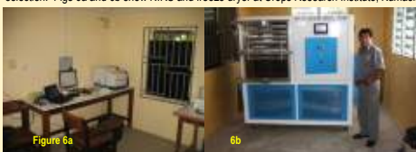
Near Infrared Reflectance Spectroscopy (NIRS) helps with the rapid analysis of samples for selection. Figs 6a and 6b show NIRS and freeze dryer at Crops Research Institute, Kumasi.
