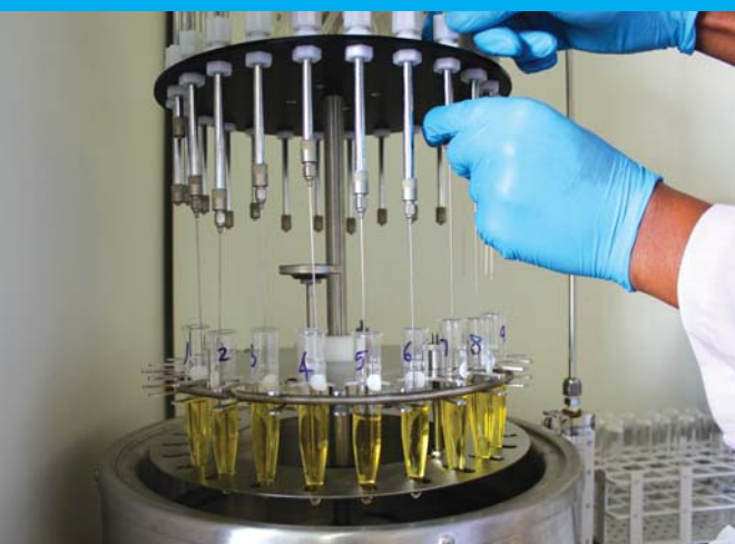
■ Fig. 2 An extract of OFSP total carotenoids in an organic solvent being dried and concentrated before analysis on a High Performance Liquid Chromatography (HPLC) system for identification and quantification. (credit S. Quinn)
