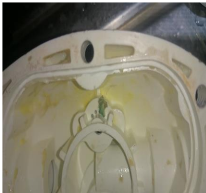
Figure 5: Improperly cleaned Equipment
