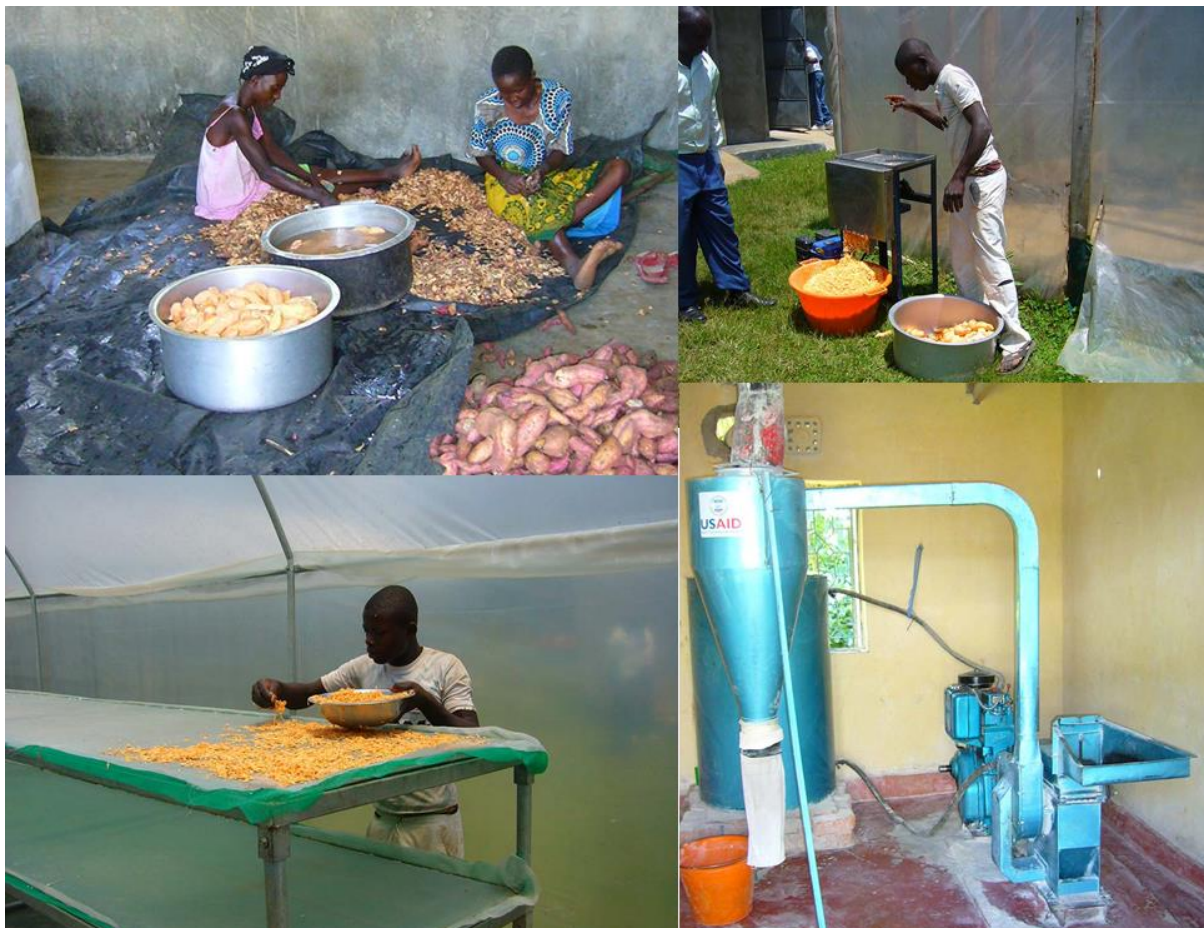
Figure B1. OFSP processing activities in Busia County: peeling of fresh roots, chipping, drying the chips and the milling machine (Photos: Ilaria Tedesco)
