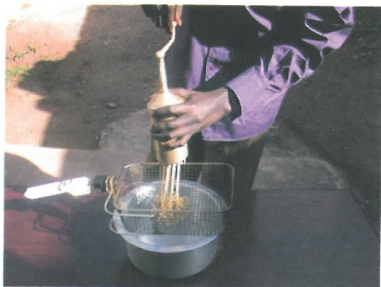
Rotate the machine to release the dough threads into a wire mesh basket
