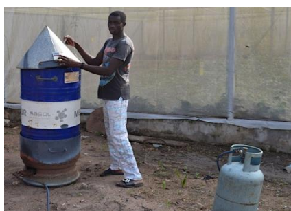
Improved barrel and LPG for soil sterilisation. The fabricated system with the lid has a slot for a thermometer to monitor temperature. Photo Credit: Boadi K. Ahenkorah
