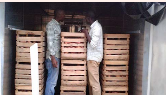
Fig. 1 Sweetpotato crates loaded into solar-powered container store at trial set-up at Organi Ltd, Home Bay County, Kenya (Credit Tanya Stathers, NRI)
