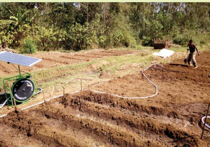
Fig 1. Solar water pump irrigation system in use with private multiplier (Credit B. Biazin)
