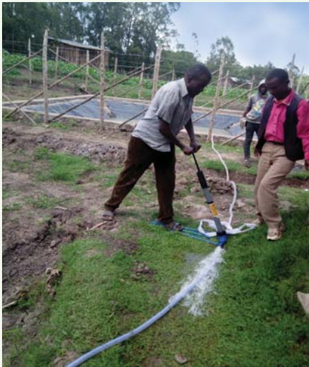
Fig 2. Water harvesting pond combined with use of a hip pump at an FTC (Credit B. Biazin)
