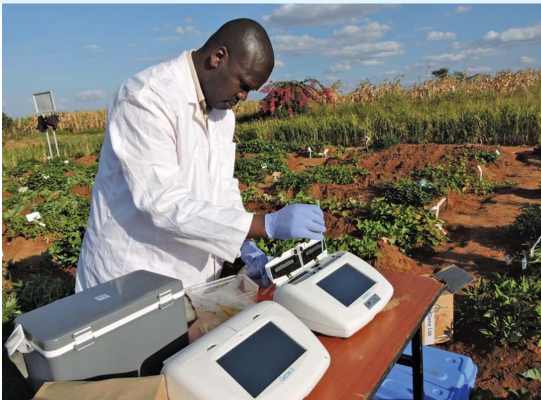
Fig. 1 Portable LAMP Genie II machine for real time detection of sweetpotato viruses in field
