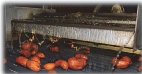
Fungicide application using a waterfall curtain
