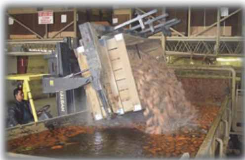
Pouring sweetpotato roots into water using a fork-lift mounted bin rotator device
