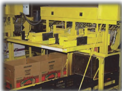
Automatic box fillers integrated into electronic sizing equipment
