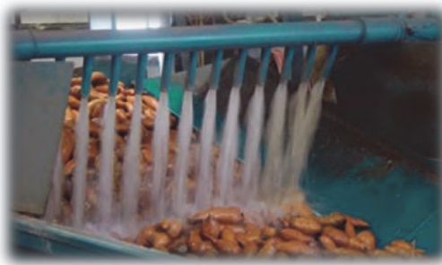
High volume water rinse used to clean sweetpotato roots
