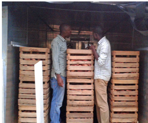
Fig. 4 Sweetpotato crates loaded into solar-powered container store at trial set-up at Organi Ltd, Home Bay County, Kenya (Credit: T. Stathers)
