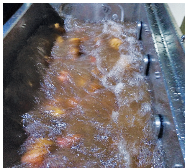
Fig 4. Washing machine can clean 100 kgs of roots in 6 minutes at Mother's Holdings (Credit: J. Low)
