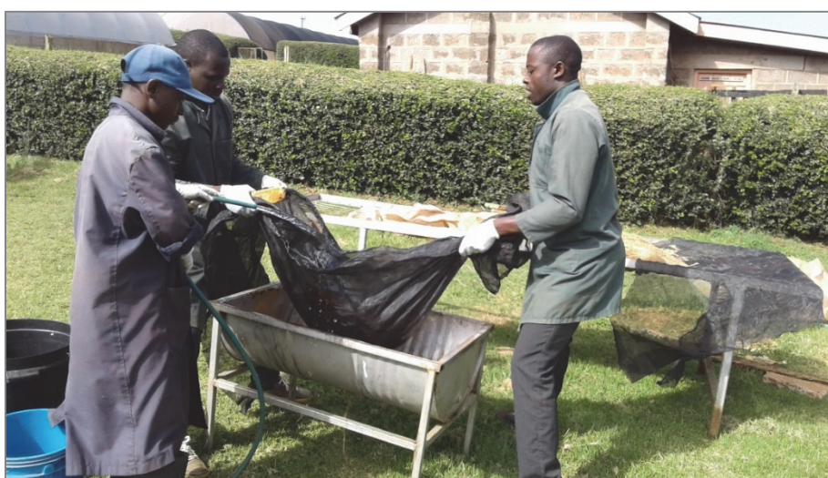
Figure 8. Washing, sterilization and drying of sand on a raised rack
